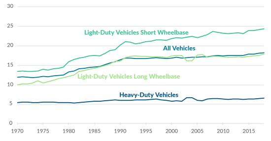
Note: Light-duty vehicle short wheelbase (WB) includes passenger cars, light trucks, vans, and sport utility vehicles with a WB equal to or less than 121 inches. Light-duty vehicle, long wheelbase includes large passenger cars, vans, pickup trucks, and sport/utility vehicles with WBs larger than 121 inches. Source: U.S. Energy Information Administration, "Motor Vehicle Mileage, Fuel Consumption, and Fuel Economy," accessed July 27, 2020, https://www.eia.gov/opendata/qb.php?category=711246.
